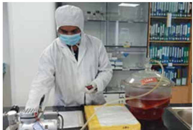
Performing Sealing Integrity Test of Medical Devices using Leak Test Apparatus
