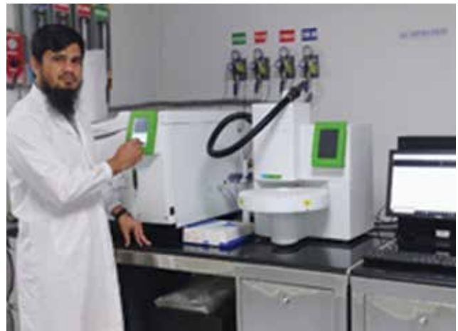
EO & ECH Residual Content Measurement of Medical Devices by Gas Chromatograph (GC)
